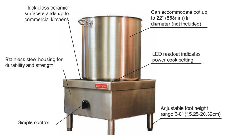
The MSP Induction Stock Pot range establishes the benchmark for high volume boil and simmer applications. Rated at 7000 or 8000 watts (depending on model), the MSP can boil a gallon of water (3.75 liters) in just 150 seconds. Five gallons (19 liters) takes just 12.5 minutes or less. With ten incremental power cook settings, an accurate simmer can then be maintained.
