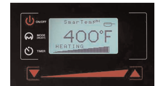
Apogee faceplate shown in temperature mode
